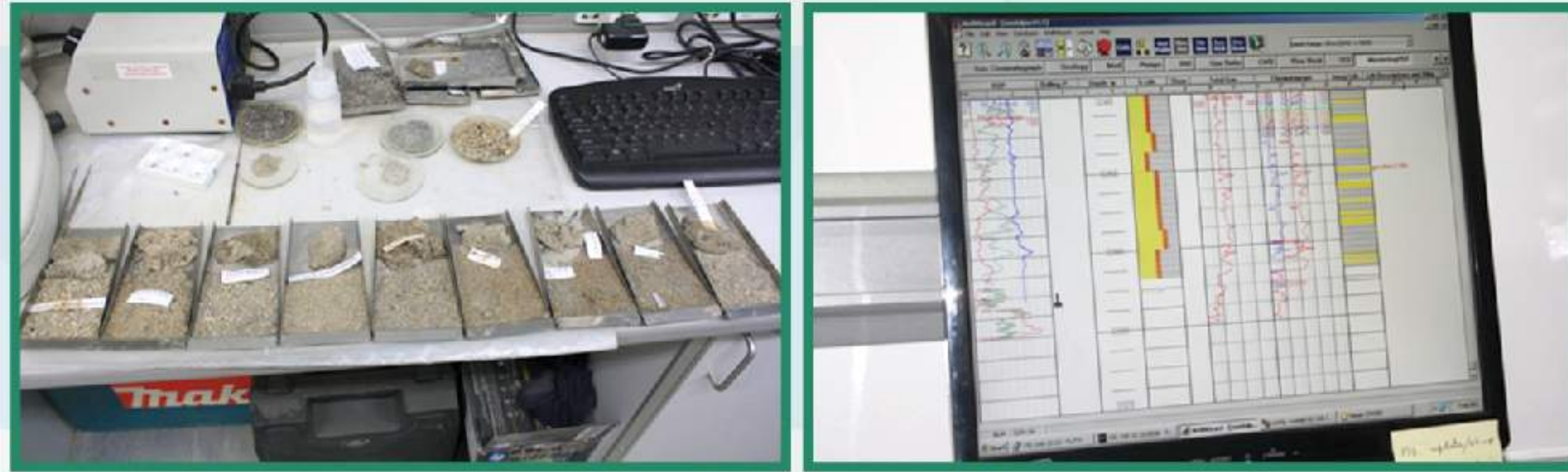
During drilling, rock samples are collected and analyzed in Mudlogging Unit to prepare a Masterlog
